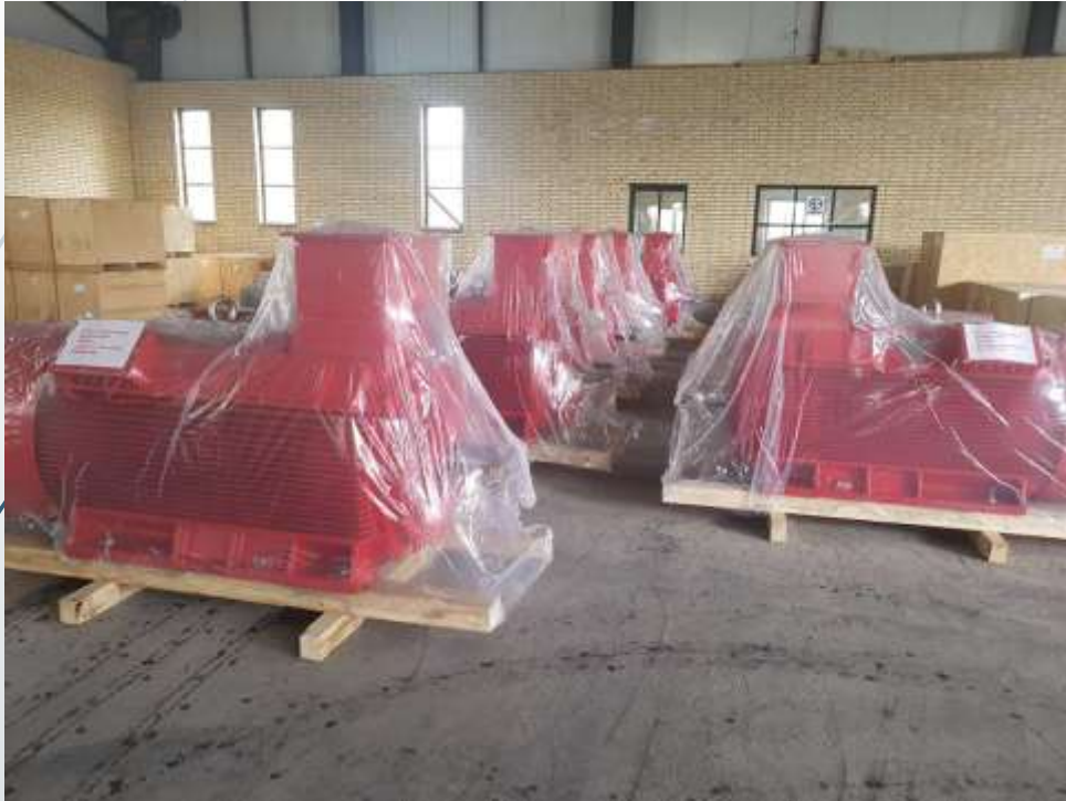
VEM motors- Kala Pump 6 pcs of 560 KW- 1500 RPM- 6000 V, 2017
