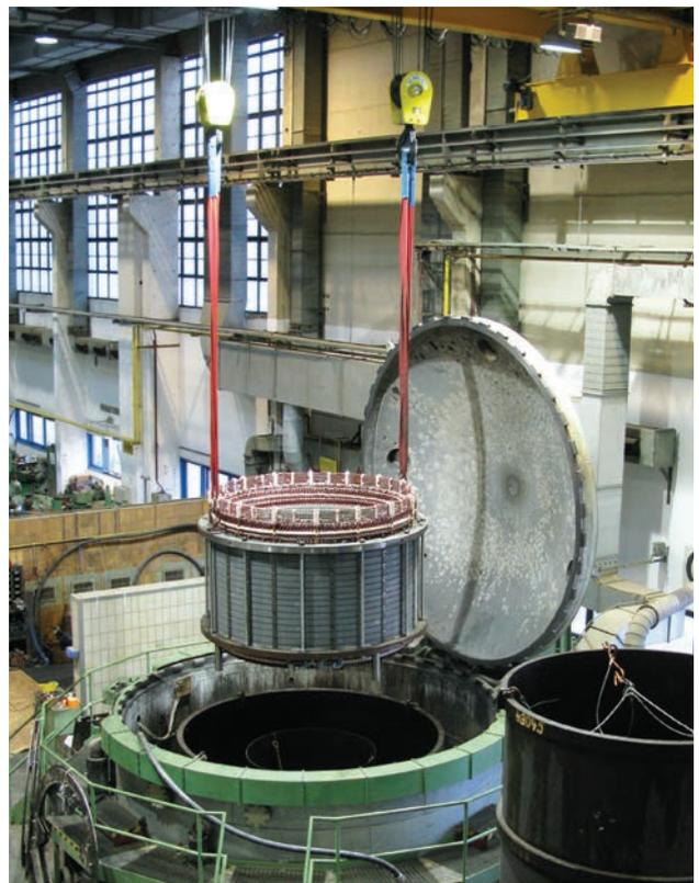
The VPI process guarantees high mechanical strength, particularly of the winding heads, as well as outstanding dielectric strength. This applies especially for breakdown voltages. Rated surge voltages in accordance with [3] are guaranteed with high certainty for all generators.
